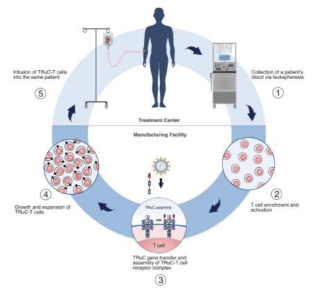
We use a next-generation cell processing platform that performs cell sample loading, cell washing, density-based cell separation, magnetic separation, cell culture and final product formulation. This is a semi-automated and functionally closed system that we believe will enable us to scale our TRuC-T cell manufacturing and overcome the constraints associated with current processes.
